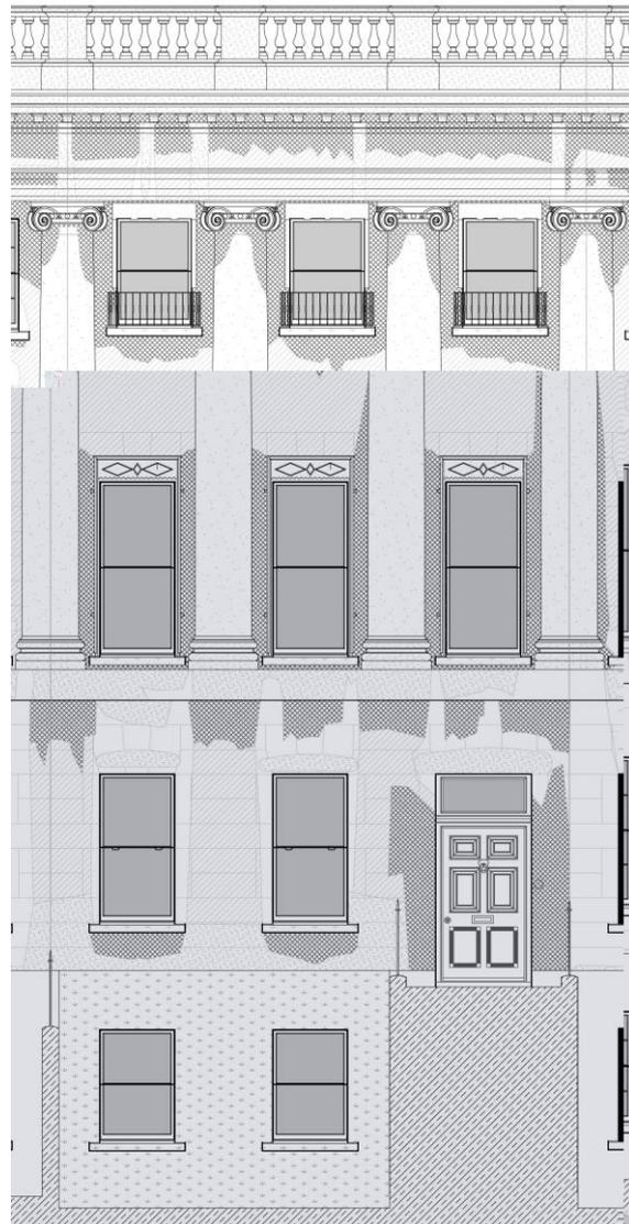
Figure 6 Typical weathering and soiling patterns
